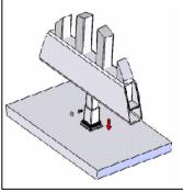
Ensure the set screw is installed through side of both sliding pieces of foot block. The screw is used to "lock" the foot block so it will not return to it's collapsed state. This step is essential for optimum porch railing performance.
