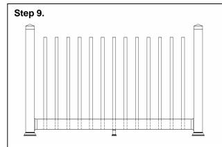
Insert pickets into bottom rail. Ensure pickets insert fully into rail and extend all the way to the bottom. Pickets will insert approximately 3% inches.
