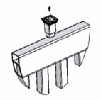
One foot block is supplied for 4, 6 and 8 foot long porch rail. Two foot blocks are supplied for 10 foot long porch rail.
