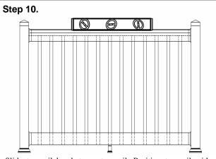
Slide top rail brackets on top rail. Position top rail with aluminum insert onto pickets. Ensure pickets insert fully into rail and extend all the way to aluminum insert (approximately 1<sup>3</sup>/<sub>4</sub> inches). Make sure top rail is level. Attach top rail to posts referring to steps 7 & 8 to attach brackets. Check your local building codes to determine the height of top rail from deck surface.
