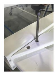
Using a 5/8" paddle bit, drill holes so that the center of the hole is over the rail. Do this for the top and bottom of the brace. Drill one hole in the center of the brace so the brace can be attached to the picket.
